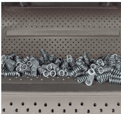
Shot peening of valve springs 970 164
