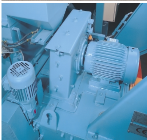
Directly driven blast wheel C 10422
