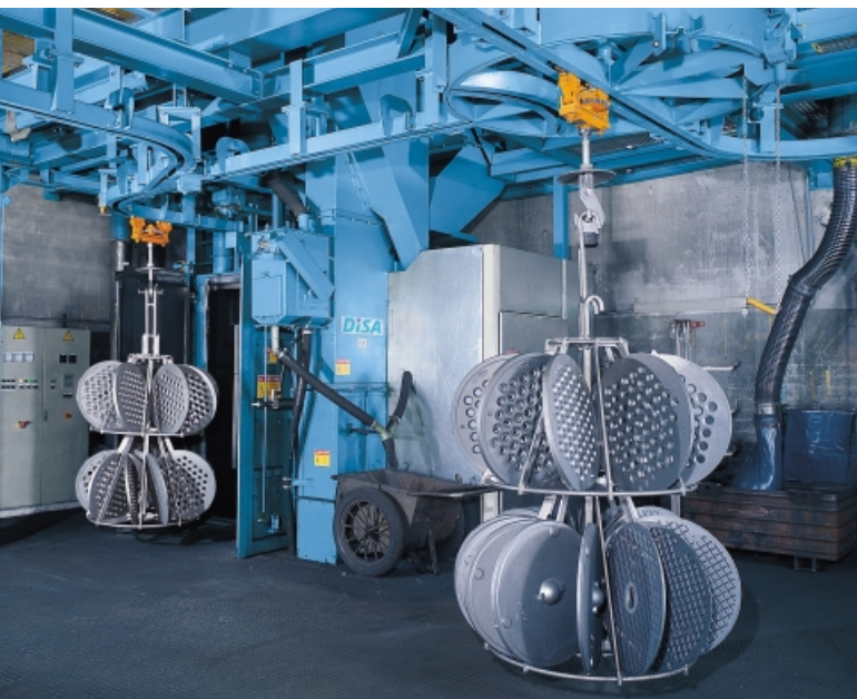
Customized monorail system with switch points turntable
