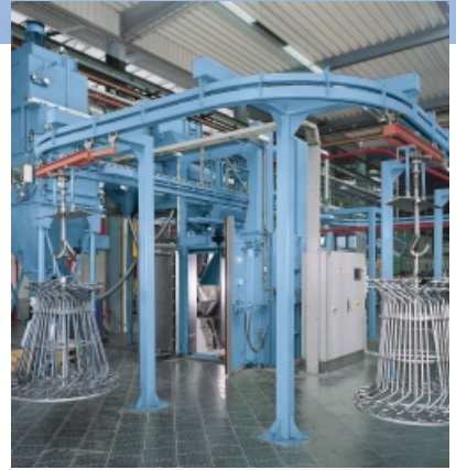
Blast cleaning system for shot peening of stabilizers for passenger cars
