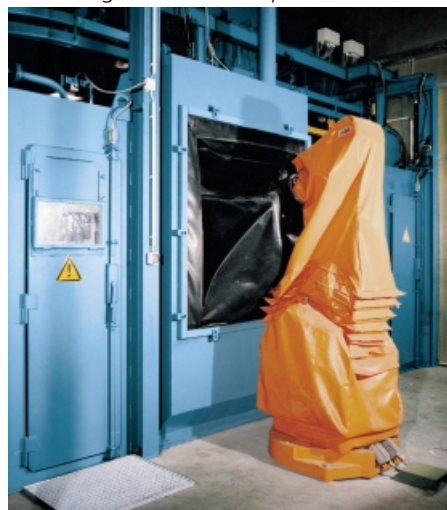
Overhead monorail blast cleaning system in combination with a robot for cleaning the inside of the parts
