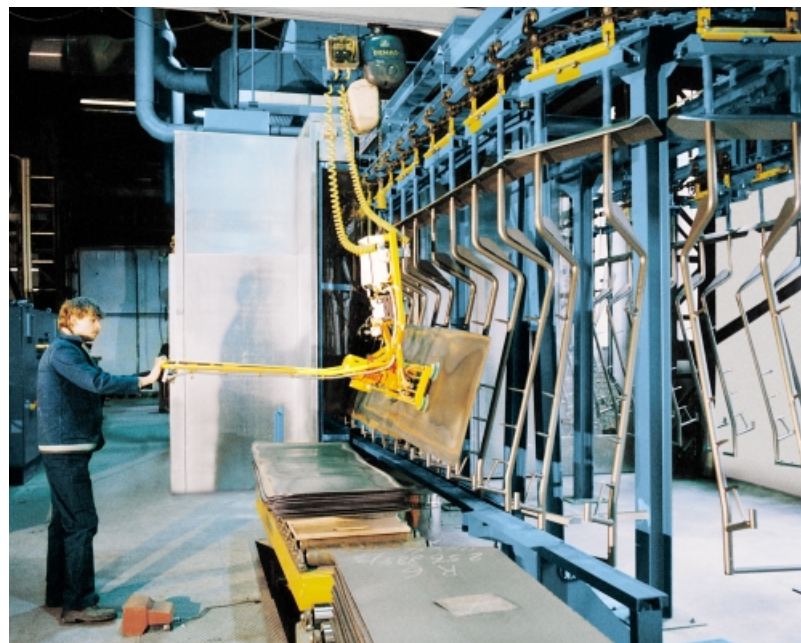
Blast cleaning system and handling equipment for blast cleaning sheet metal plates
