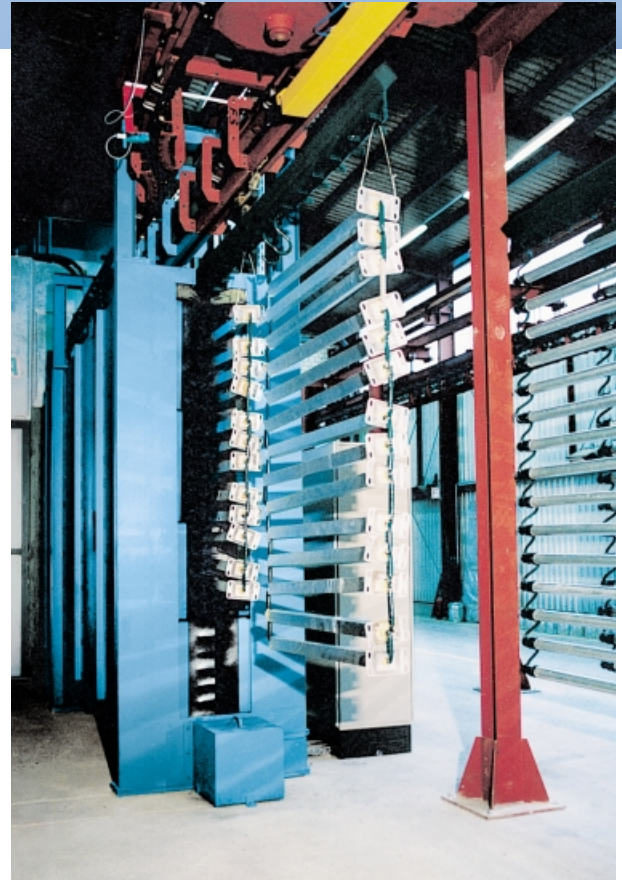
System for blast cleaning grid fences and gate components on a Power and Free system 013167
