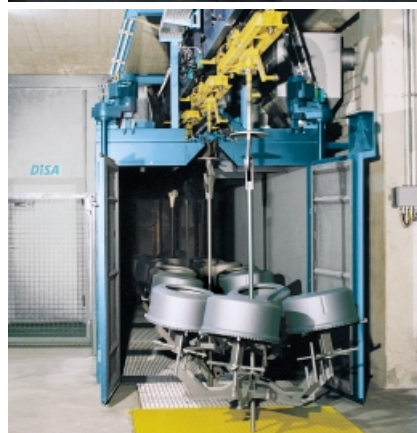
Blast cleaning of brake drums and brake disks 013166
