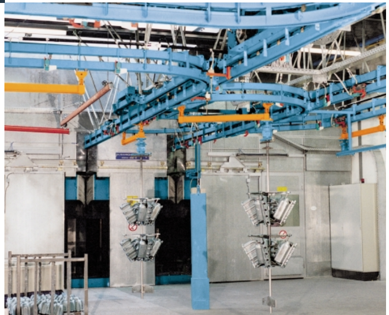
Blast cleaning of aluminium parts on a Power and Free system
