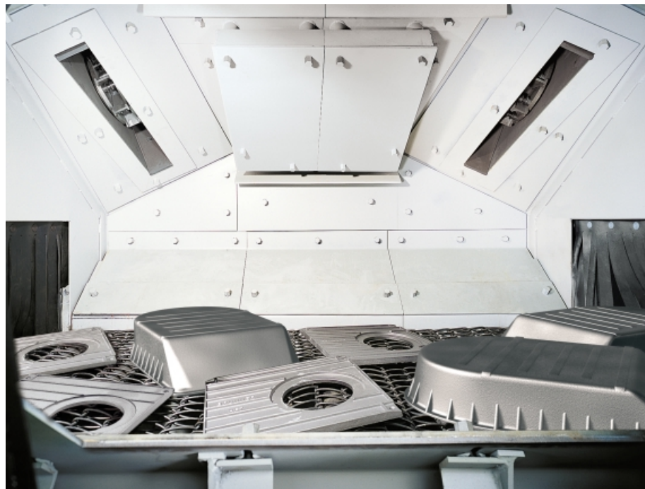
Wear resistant material is used for the blast chamber
