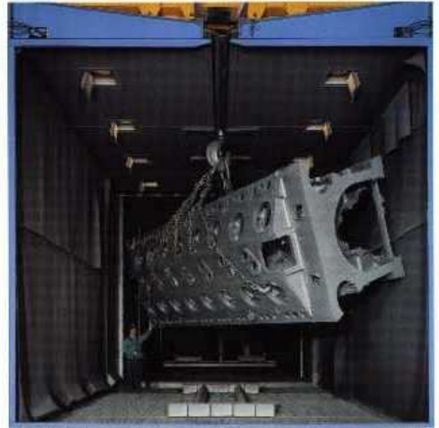
Shot blast chamber for large castings
