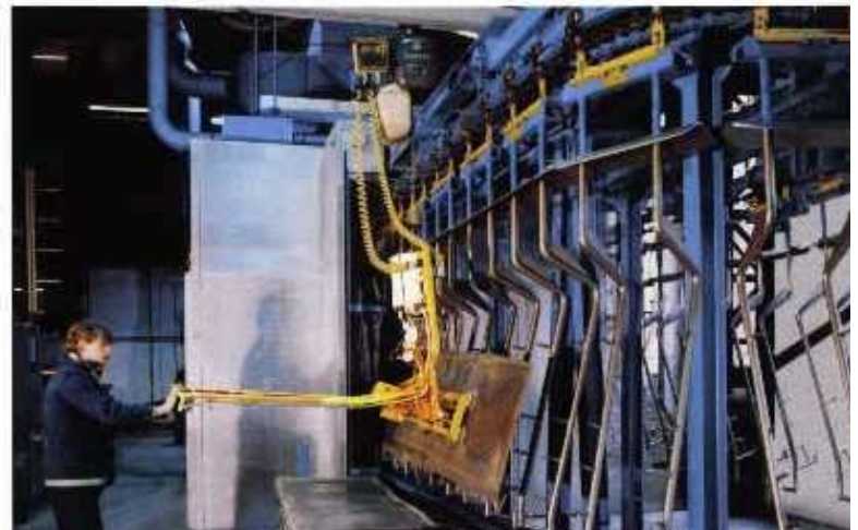
Blast cleaning system and handling equipment for blast cleaning sheet metal plates 610077
