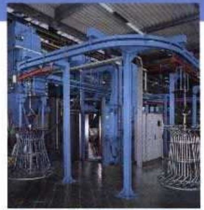
Blast cleaning system for shot peening of stabilizers for passenger cars C 9964
