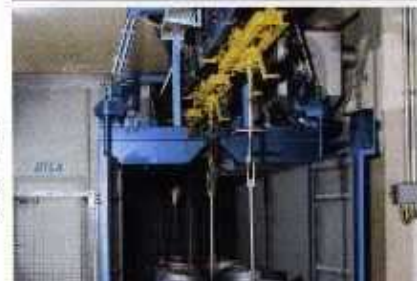
Blast cleaning of brake drums and brake disks 013166
