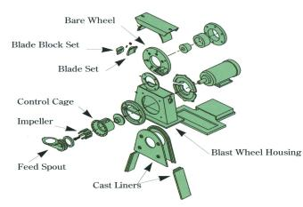
The adjustable control cage assures accurate blast pattern control.
