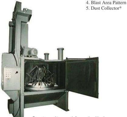
Featuring a cabinet notch for overhead loading, the DISA Goff 72" S Table Blast machine handles load capacities up to 6,000 lbs.
